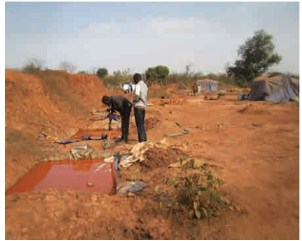
Traditional gold washing site (crushing machine and cyanide hole to harness gold) (Photo: AMCFE, 2013)
